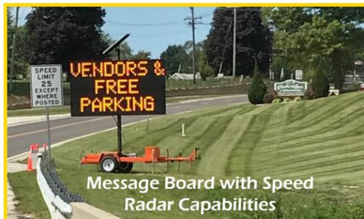
Message Board with Speed Radar Capabilities
